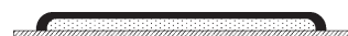
Scheme 1 Schematic representation (disk-like model) of the cross-section of a surface micelle of F8H16 after transfer of the monolayer onto a silicon wafer. The black area represents the fluorinated segment F8 region and the dotted area represents the hydrogenated segment H16 region.
